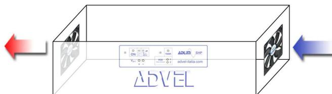
The two fans are placed so that the airflow is directed as shown in the figure:
